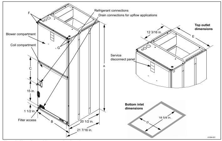
Figure 3: Dimensions and duct connection dimensions
