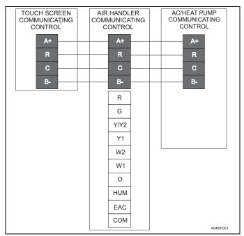
Figure 13: Air handler with communicating AC or HP
