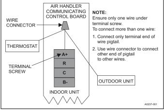
Figure 14: Multi-wire terminal connection
