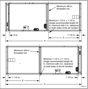
Figure 6: Suspension support locations for horizontal applications
