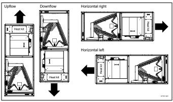
Figure 4: Typical installation
