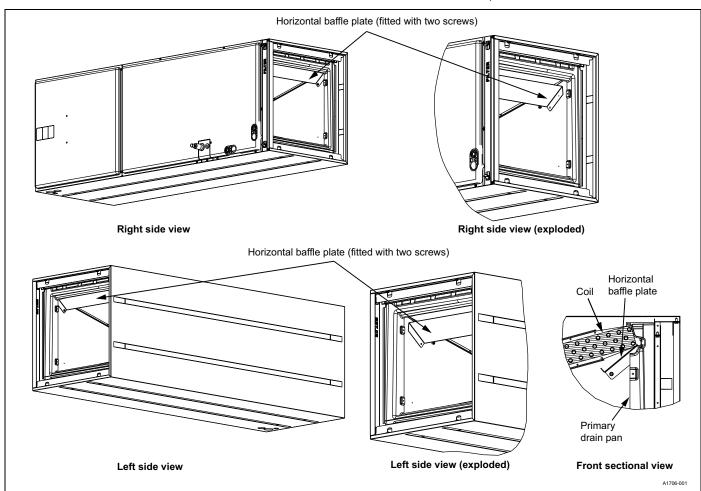
Figure 5: Horizontal baffle plate installation
