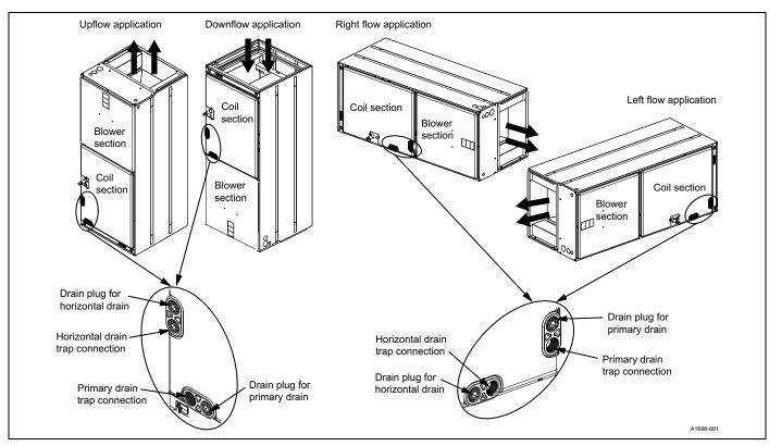
Figure 21: Location of coil trapped and plugged drain connections
