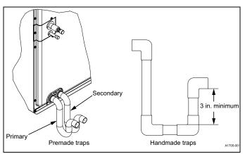
Figure 20: Drain traps
