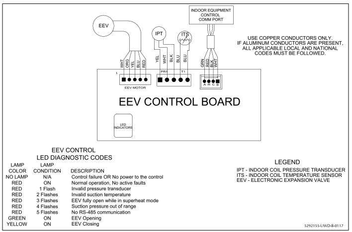
Figure 22: Wiring diagram - EEV
